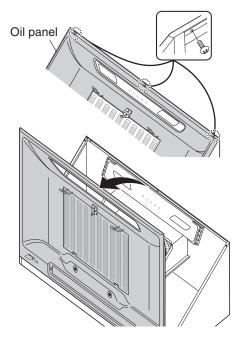
3) Using the patterned paper included, insert the washer-head wood screws (∅5.1×45) 5mm into the mounting wall for the left and right keyholes of the mounting bracket.
