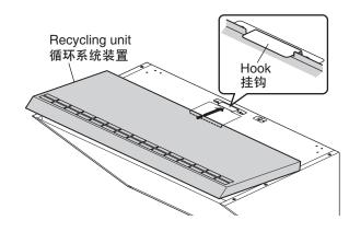
Using the holes (four locations) inside the main unit at the positions indicated by the illustration below, affix the recycling unit to the main unit with the truss screws provided.
