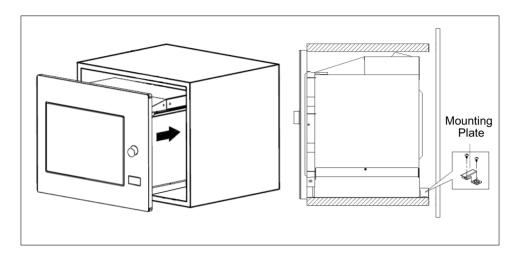
5. Use the sucket to open the door, fix the oven to the cabinet with Screw, at the installation hole.
