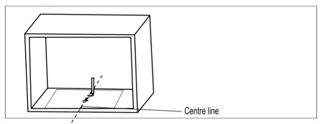
3. Remove the bottom cabinet template and fix the mounting plate with screw.
