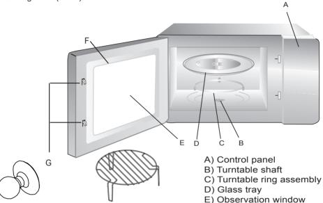
Sucker Grill Rack( Can not be used in microwave function and must be placed on the glass tray )
